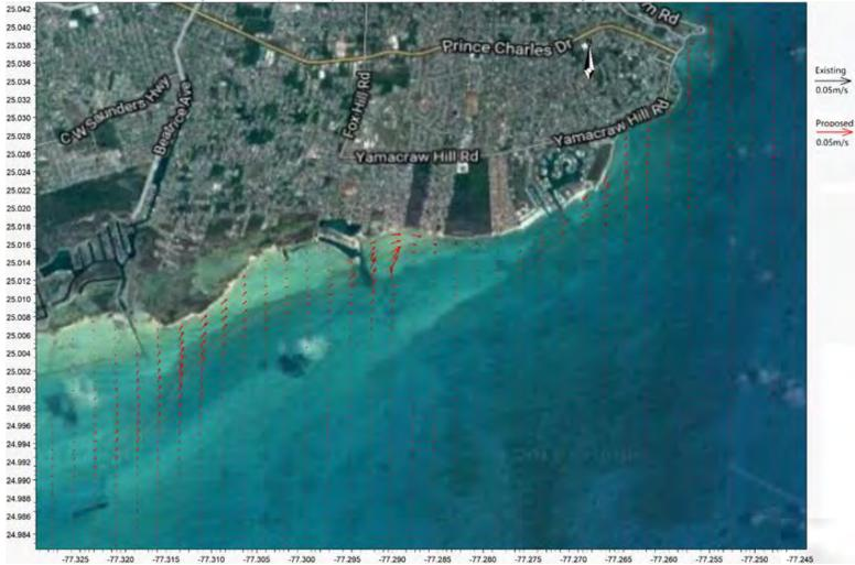
Figure 31. Comparison of Nearshore Current Velocity Vectors during South Waves.
