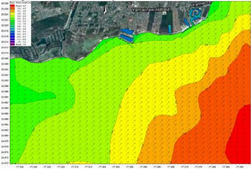
Figure 23. Wave Height Distribution for the 100-Year Hurricane Waves due to SW Wind
