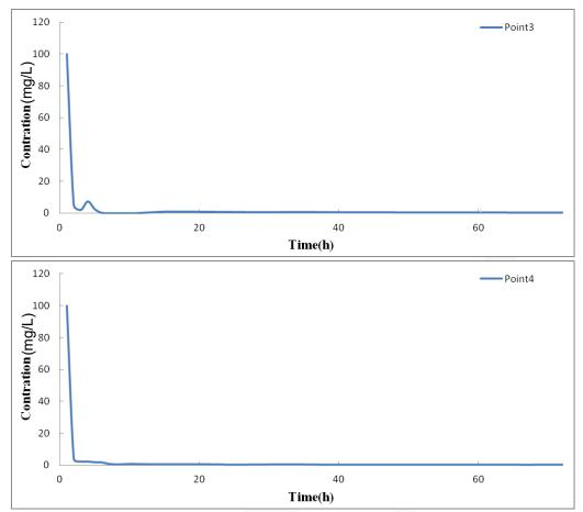
*Figure 6-9* Time series of tracer concentrations for Cases 3 (Upper) and 4 (Lower) at sampling points where the greatest tracer concentration was observed.
