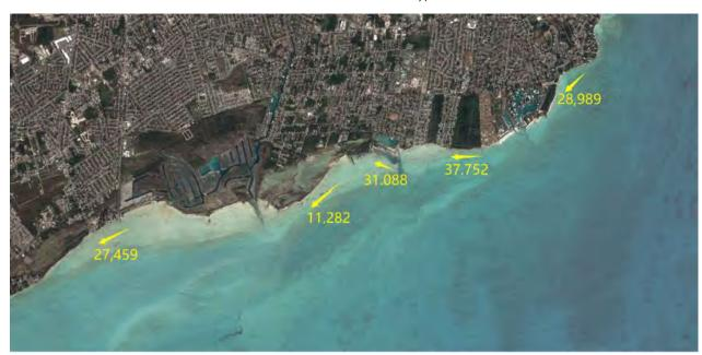
Figure 32. Long-term Annual Potential LST Rates for Existing Condition. (Note, actual LST less than potential LST due to limited sand availability)
