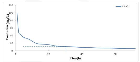
*Figure 6-7 Time series of tracer concentrations for Case 2 at sampling point 2 where the greatest tracer concentration was observed.*
