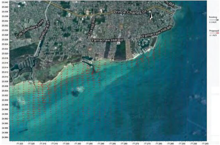
Figure 29. Nearshore Current Velocity Vectors during East Waves.
